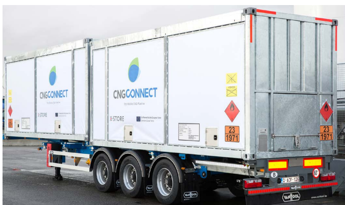
These 20 ft X-STORE containers have been sourced by Drive Systems and will be used to transport gasified LNG from mother to daughter stations.
