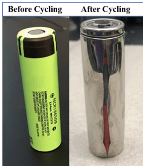
Credit: Ozkan Lab/UCR After 60 fast-charge cycles EV batteries begin to deteriorate. In some cases, cells cracked and exposed their internal components.
