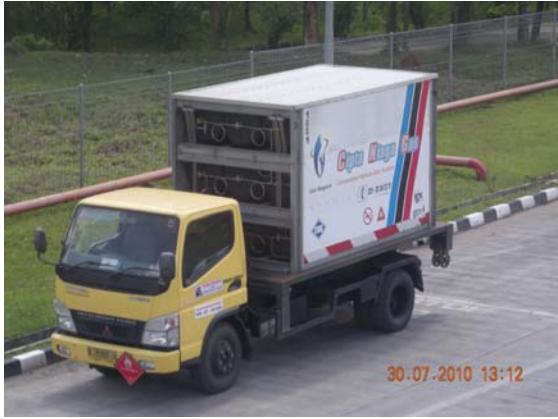
Different sizes of trailers delivering CNG from Mother Station
